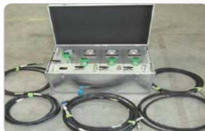
Check Fuel Tank / Line Leakage
