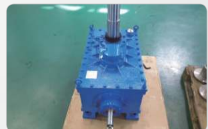
COOLING TOWER REDUCER
