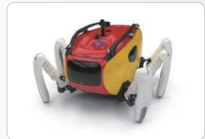
Subsea Robot Multi-joint submarine walking robot
